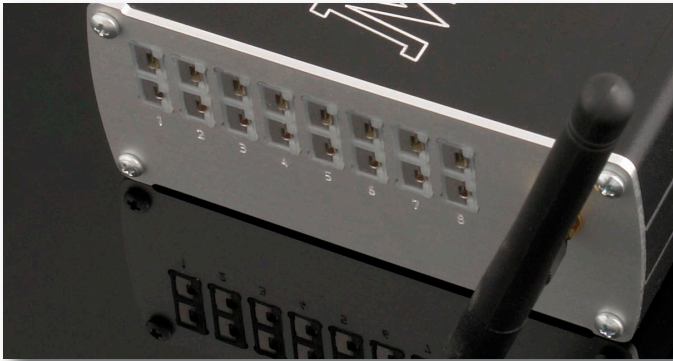
Fig 5.2.7b - On the side of the MaxxECU device you can connect the exhaust temperature sensors.
