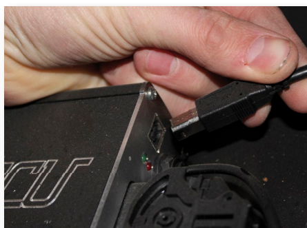
Fig 4.2.2c - Connect the supplied USB cable to the USB port on your MaxxECU device. Always try to keep the USB cable attached, mounted in the MaxxECU device for future use!
