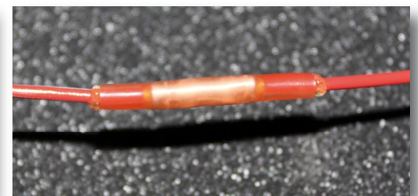
Fig 3.1.2c - Finished cable joint. There should be no burns on the cable, and glue should protrude past the ends.
