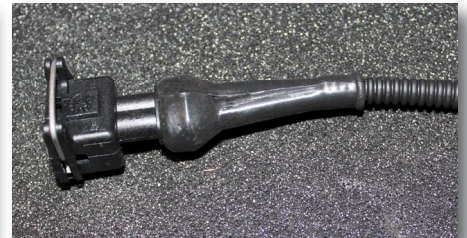
Fig 3.1.4f - Cover over with protective rubber and dress cable with slotted protector tube.
