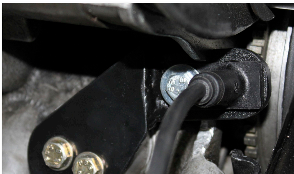
Fig 5.1.5a - Custom-made trigger attachment for bosch crankshaft sensor on a porsche 911.
