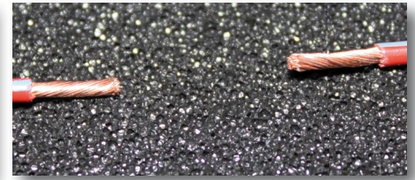
Fig 3.1.1c - The cable ends stripped and twisted together to not "splay" apart.
