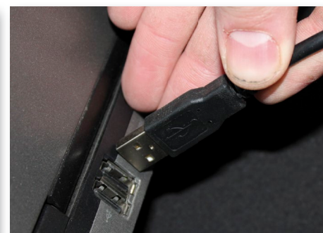
Fig 4.2.2d - Connect the USB cable from MaxxECU to your computer's USB port. Remember to always connect to the same USB port on the computer you use to MaxxECU. Windows do not always recognize the USB connected devices if they are connected on ports other than the one used when the driver was installed.
