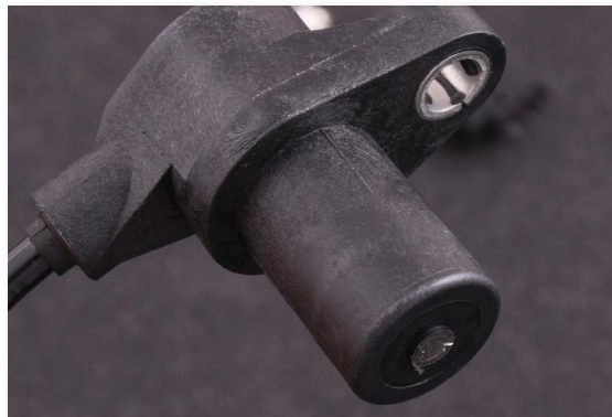
Fig 5.2.0b - Bosch trigger sensor (VR)
