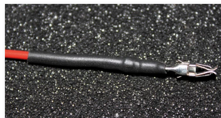
Fig 3.1.5e - A finished cable bonding that has been done with soldering.
