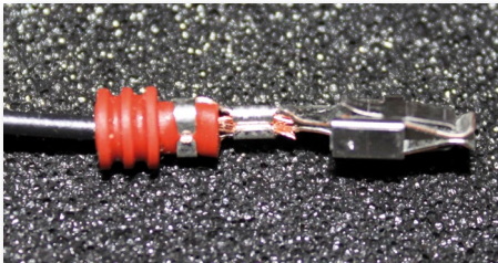
Fig 3.1.4d - A good bonding, pin both isolation (strain relief) and the electrical conductor.
