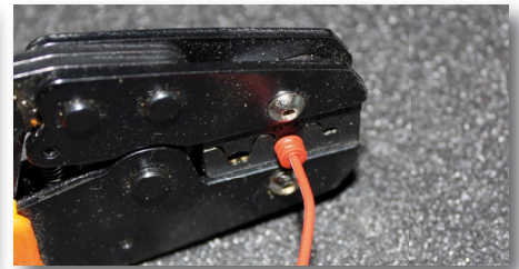
Fig 3.1.4c - Thread the cable with the seal in the cap and crimp with a quality crimp tool.
