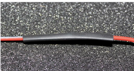
Fig 3.1.3d - Pull the shrink tube and place it over the center of the joint.
