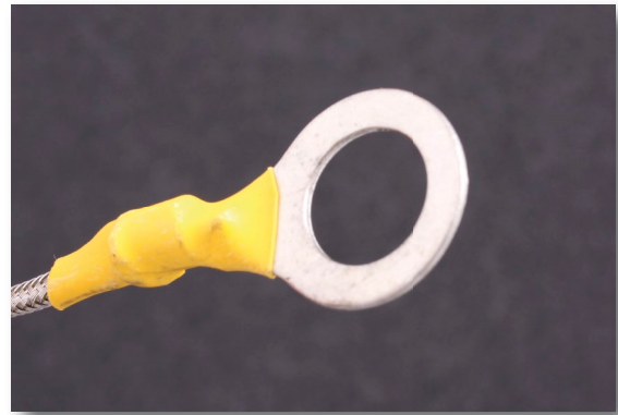
Fig 5.2.0f - Temperature sensor for mounting on eg gearbox, diff or engine blocks. Type-k.
