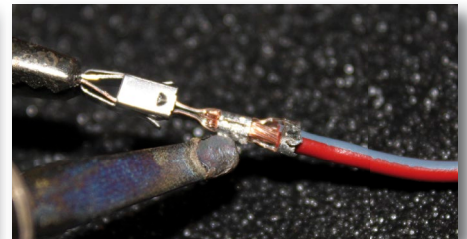
Fig 3.1.5c - Heat up the pin with a heat gun and add the solder, melt together.
