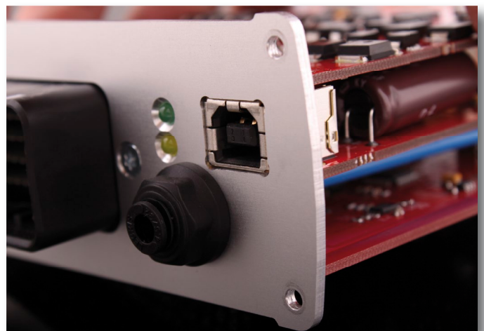
Fig 1a - MaxxECU control electronics, without protective cover.
