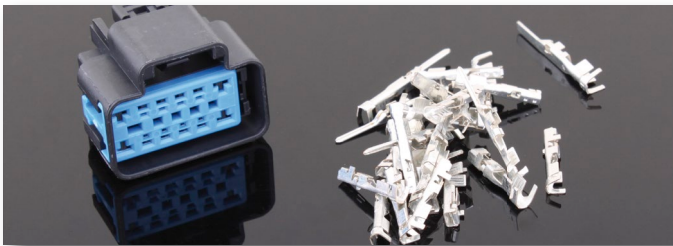
Fig 4.1.2c - 12-pin connector for connecting the power supply, buttons, warning lights, tachometer and such. Even MaxxECUs power should go through this connector! The idea behind this "extra" connector is that in principle we should be able to release the two connectors [this and the 48-pin Molex connector] and then be able to "lift the engine incl harness" without cutting any wires.
