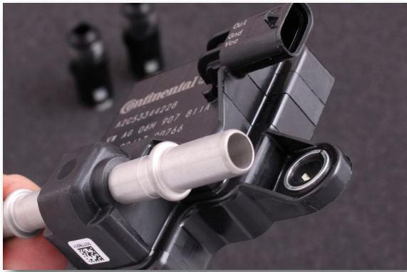
Fig 5.2.0e - Digital ethanol sensor for reading the fuel temperature and ethanol concentration.
