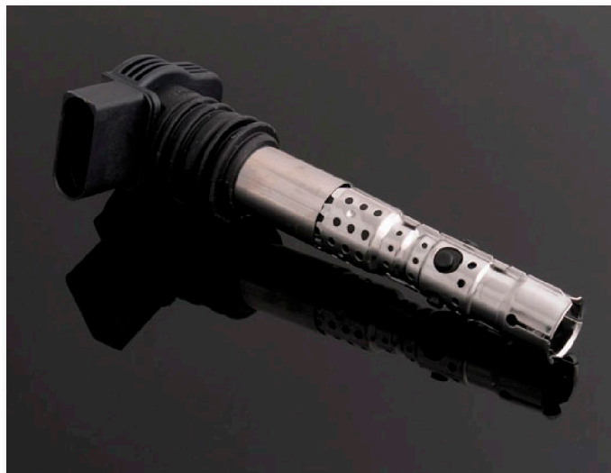
Fig 6.1.1b - VAG coil is often used because they are relatively cheap and good ignition coil with built-in module which means you do not need any external electronics between coil and MaxxECU.
