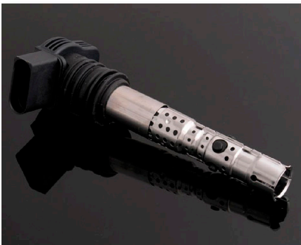
Fig 6.1.2b - VAG ignition coil has built-in interference suppression and is a good option for most engines where it is possible to mount it directly on the spark plug. Three different lengths of the coil is available to suit most engines.
