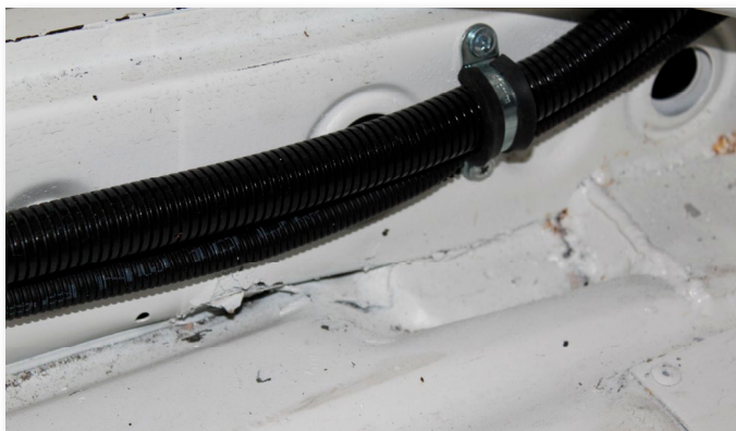
Fig 3.2.1g - Examples of the use of corrugated tube and tape. The installation is more attractive and safe!
