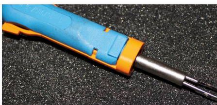
Fig 3.1.6a - Tool to safely remove contact pins without marring the connector.
