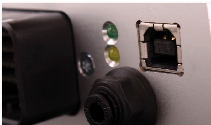
Fig 4.3.2c - MaxxECU has two indicator LEDs on the side of the connector.
