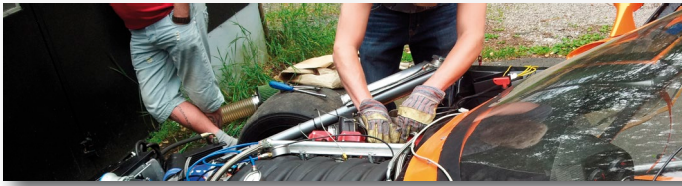
Fig 7.2.1i - Attempt to start the engine, note to avoid voltage drops below 8v to MaxxECU (communication ceases). Enable logging for future troubleshooting if the engine does not start at this stage.
