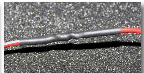
Fig 3.1.3f - A good, sturdy, solder joint with heat shrink tubing looks like this!
