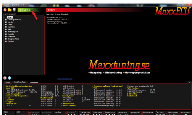
Fig 4.2.2e - Windows will detect when MaxxECU is connected and thus can find the device without MaxxECU is powered, however, no form of communication will occur before MaxxECU is powered by turning on the ignition. When the ignition is on, MTune indicate that communication exists by changing the status text to "ONLINE" instead of "OFFLINE" in the upper left corner of MTune!
