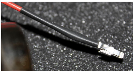
Fig 3.1.5d - We recommend using heat shrink tubing with glue! in this case to protect, cover and heat with a heat gun.
