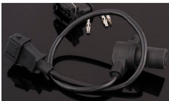
Fig 5.1.2b - Examples of VR sensor and its wiring.
