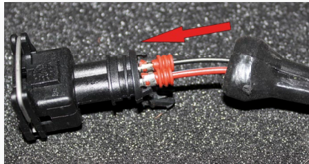
Fig 3.1.4e - Insert the contact pin in the electrical connector until you hear a "click". The pins should not be pressed in with force.
